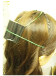
Fig. 2. Accelerometers mounted in the occipital region.
